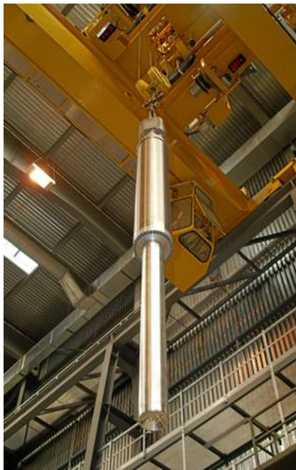
Fig. 2. The fully assembled MEGAPIE target before being inserted into the SINQ operation position.
